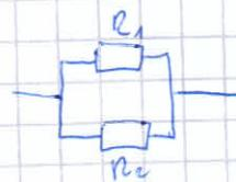
$$R_{\text{el}} = \frac{1}{R_{\text{el}}} = \frac{1}{R_1} + \frac{1}{R_2}$$
