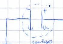
$$C(V_2 - V_1) = q$$
