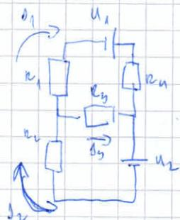
$$\begin{aligned} I_1 + I_3 - I_2 &= 0 \\ I_1 &= I_1 R_1 - I_3 R_3 + I_2 R_2 \\ -U_2 &= I_2 R_2 + I_3 R_3 \end{aligned} \quad \left. \begin{array}{l} \\ \\ \end{array} \right\}$$
