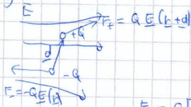
$$F = Q \underline{E}(n+d) - Q \underline{E}(n) = Q [\underline{E}(n+d) - \underline{E}(n)] = *$$
