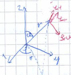
$$dr = dr \underline{e}_r + r d\alpha \underline{e}_\alpha + r \sin \alpha d\phi \underline{e}_\phi \quad (2)$$
