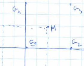
$$G_1 = \begin{pmatrix} 0 \\ 0 \end{pmatrix}, \quad G_2 = \begin{pmatrix} \frac{2\pi}{a} \\ 0 \end{pmatrix}, \quad G_3 = \begin{pmatrix} \frac{2\pi}{a} \\ \frac{2\pi}{a} \end{pmatrix}, \quad G_4 = \begin{pmatrix} 0 \\ \frac{2\pi}{a} \end{pmatrix}$$
